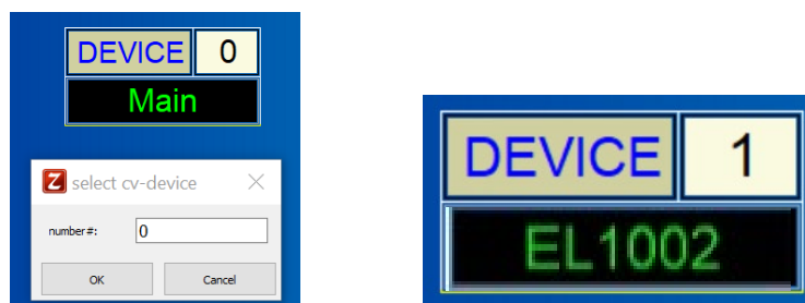
Fig. 4: Selecting an external potentiostat in the test sampling window. DEVICE 1: EL1002 indicates that the EL1002 is connected to the port 1 of the EPC42 card.
