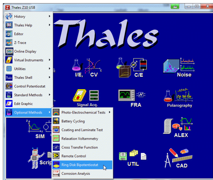
Figure 3: The RD software panel is opened by means of the pull down menu.
