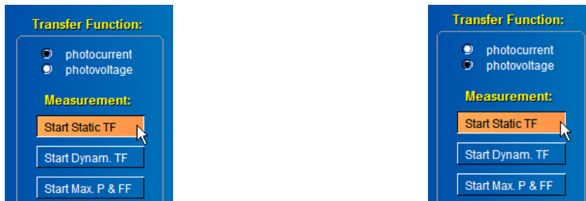
Fig. 31. Entry buttons for the measurement of the DC photo-current- (left) and DC photo-voltage characteristic (right).
