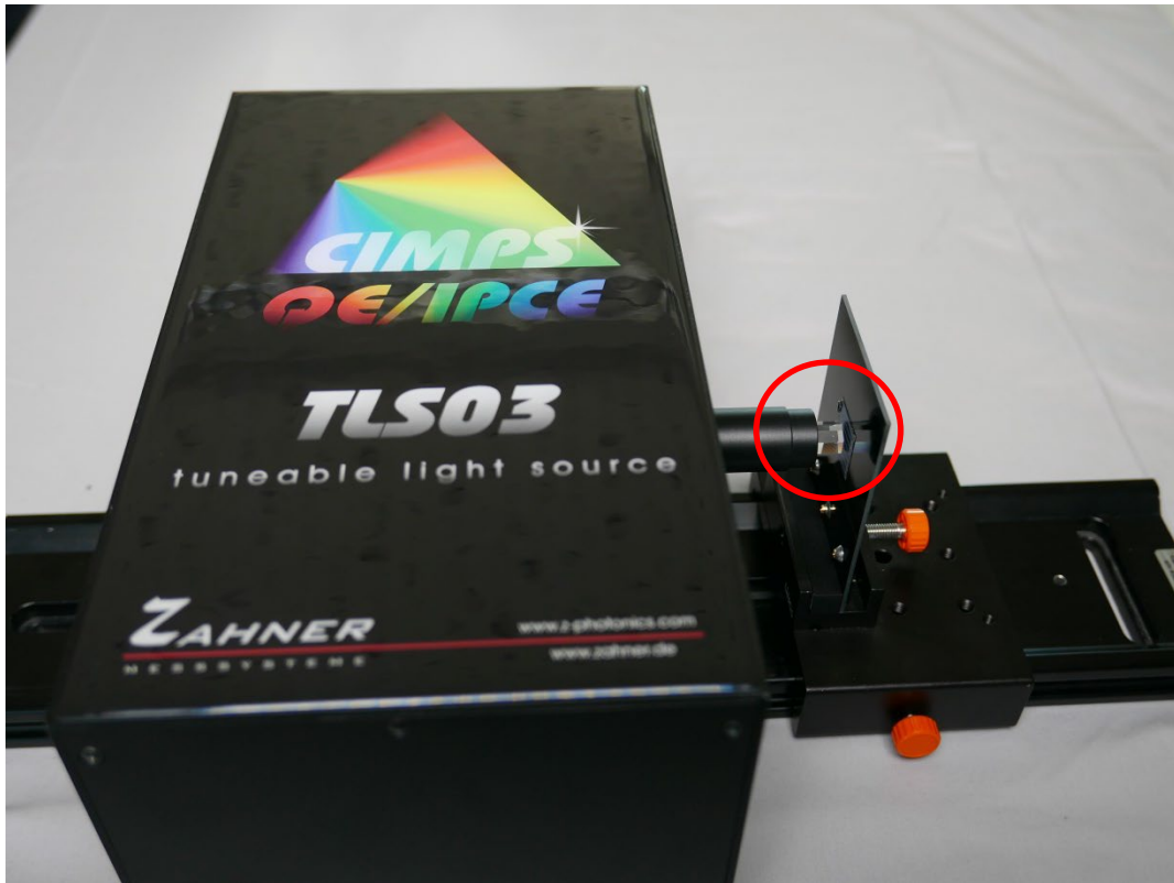
Fig. 3: Correct positioning of the solar cell relative to the TLS03. The optimal distance between the light guide of TLS and the solar cell is ~1 mm.
