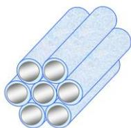
Figure 4. Porous, hexagonal structure of the parent silica material
