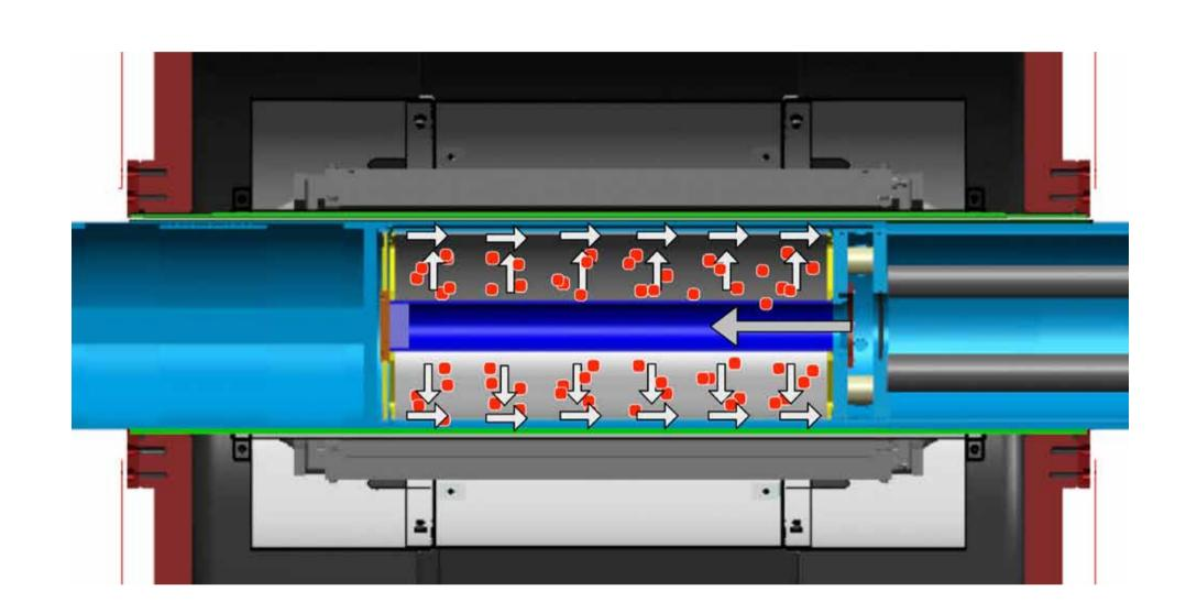
The SHGMS has a room-temperature horizontal bore of 8" (203mm) with an effective processing space length of 16" (406mm). Over this cylindrical volume the superconducting magnet produces an average of 5 T flux density with variation of less than +/- 10%.
