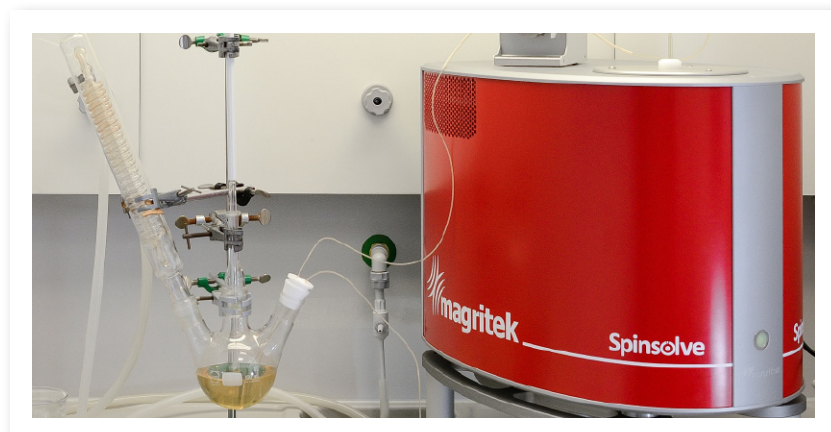
Hydrolysis of acetic anhydride with mass balance (see Magritek Application Note 9)
