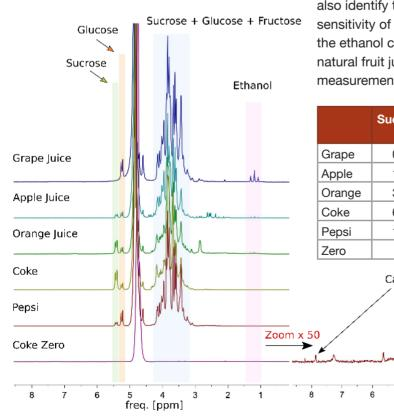
Spinsolve ULTRA measures not only the sugar content but can also identify the type of sugars present in the sample. The high sensitivity of the system allows you to quantify with high accuracy the ethanol content typically present at very low concentrations in natural fruit juices. The samples here are all neat. All measurements took 8 minutes, except Coke Zero was 1 hour.
