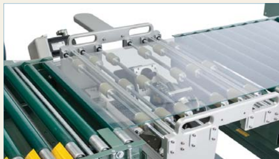
In-Line ellipsometer measuring a film through a glass panel.
