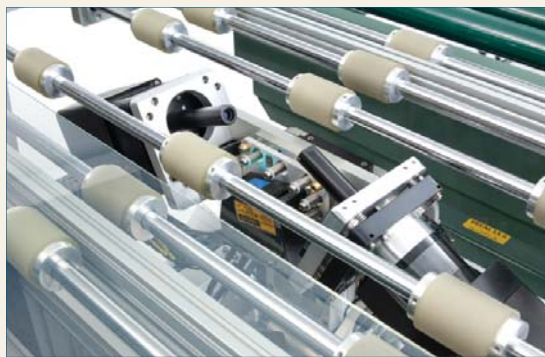
Close-up of an In-Line ellipsometer integrated within a conveyor system.
