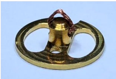
Fig. 3: 3D puck calibration fixture, showing the copper braid extended to optimize the contact area made with the calorimeter platform.
